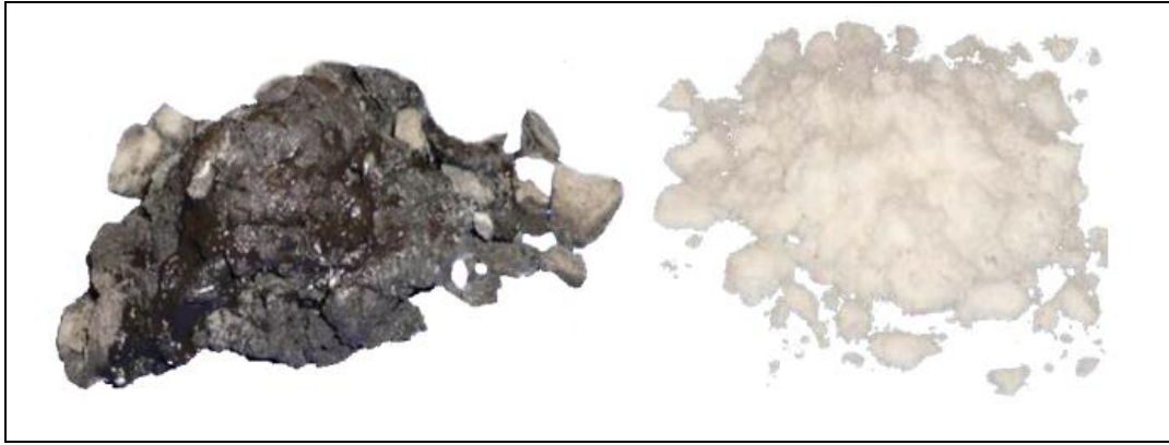
Figure 2-28: (a) Hydrocarbon contaminated salt cake (b) Clean Salt Cake [64]
