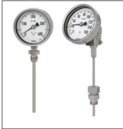
Figure 3-12: Bimetal thermometer (Top of the column) [97]
