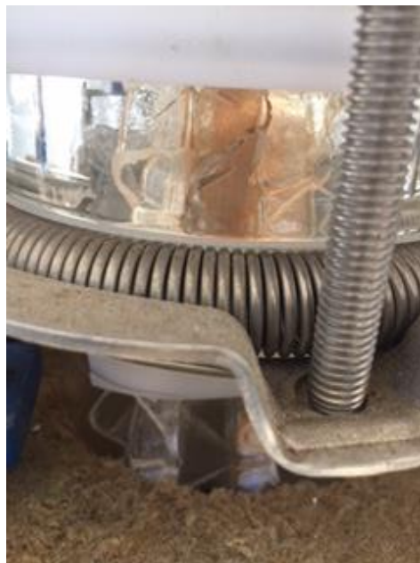
Figure 6-12: Scale formation on the packed bed column
