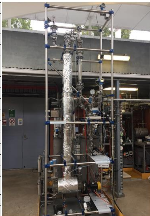
Figure 4-3: MEG Distillation Column [118]
