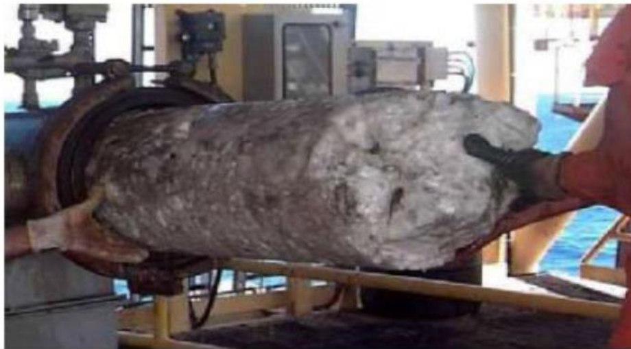
Figure 1-1: Hydrate formation in natural gas transmission pipeline [6].
