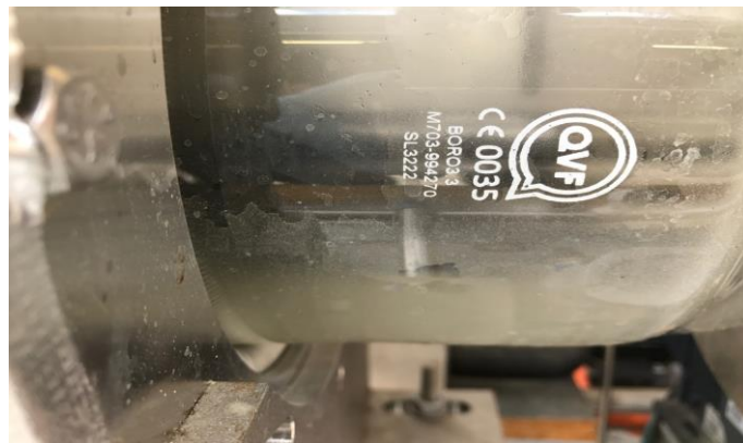
Figure 6-11: Scale formation on the reboiler glass vessel
