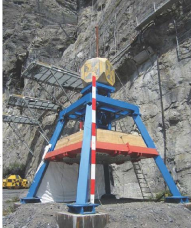
Figure 2.20. The large-scale dynamic testing rig of Geobruigg (Roth et al., 2014)
