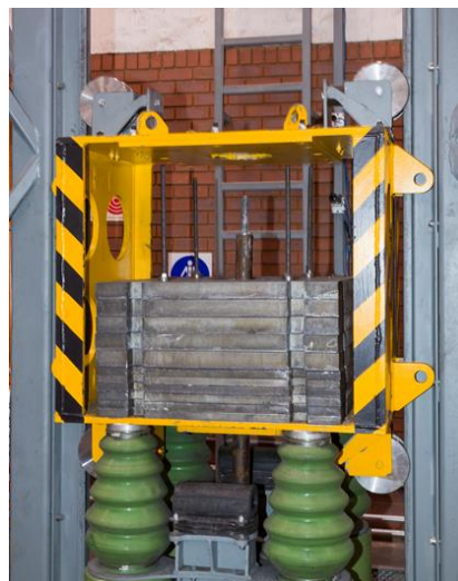
Figure 2.21. The New Concept Mining (NCM) Dynamic Impact Tester (DIT)
