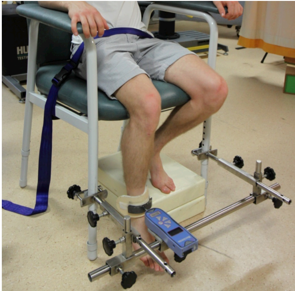
Figure 3-2 Position of participant and dynamometer for measurement of the strength of the knee extensors
