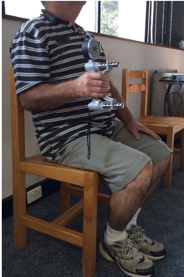
Figure 3-5 Position of participant and dynamometer for measurement of the strength of hand grip
