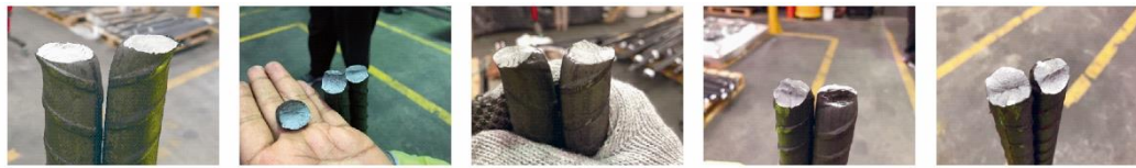
(a) 20 mm (b) 30 mm (c) 40 mm (d) 50 mm (e) 60 mm Figure 3.27 – Rockbolt surfaces after failures for SA M24.
