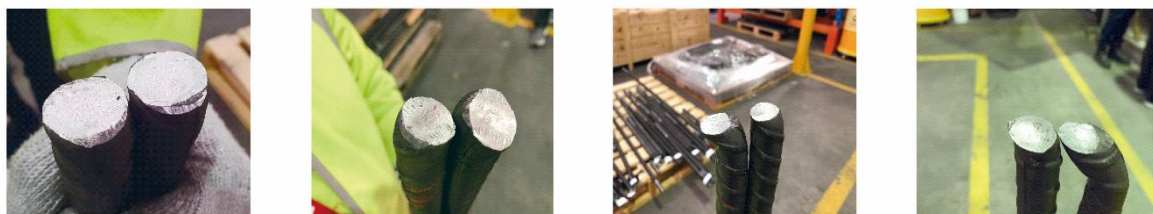
(a) Pure shear (b) 5 mm (c) 10 mm (d) 15 mm Figure 3.16 - Failure mechanism of rock bolts with/without a gap.
