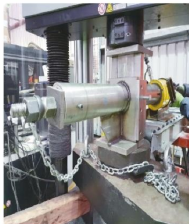
Figure 3.7 – Combined Load set up test.
