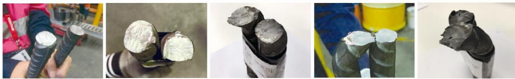
(a) Pure shear (b) 5 mm (c) 10 mm (d) 15 mm (e) 20 mm Figure 3.15 – Failure mechanism of rock bolts with/without a gap.
