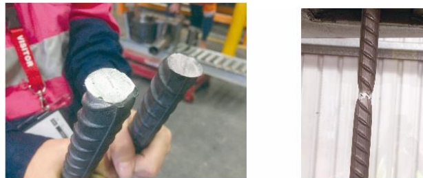
(a) Shear tests failure profile (b) Tensile tests failure profile
