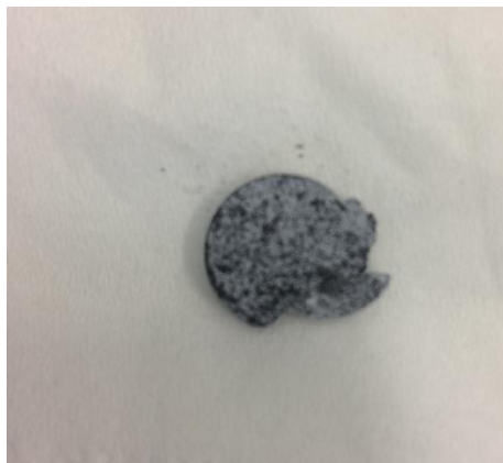
Figure 5.10 Defective surface of the composite membrane with the mixed layer of 80% zeolite pressed at 8 MPa for 2 minutes.
