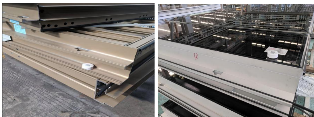
Figure 6: A smart sensor attached to a façade panel
