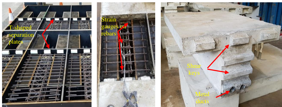
Figure 2-3: Casting of specimens
