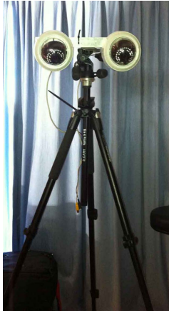
Figure 15. Side by side cameras. Both images were in same viewing plane and provided no depth of field benefit.
