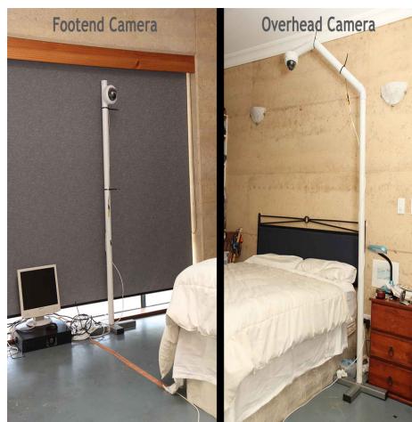
Figure 17. Foot end and side overhead. The combination of an overhead camera and foot end camera, provided both the optimal viewing angles for depth of field and practical placement in the majority of homes. Cables were secured to flooring in areas of foot traffic for safety.
