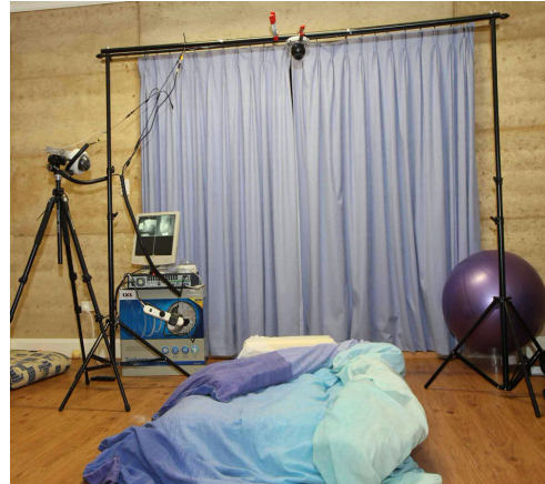
Figure 16. Side and overhead cameras. To obtain improved depth of field camera viewing, visual planes were orientated 90 degrees to each other. However, in this setup lack of room and safety when exiting the bed at night made a side camera position impractical.
