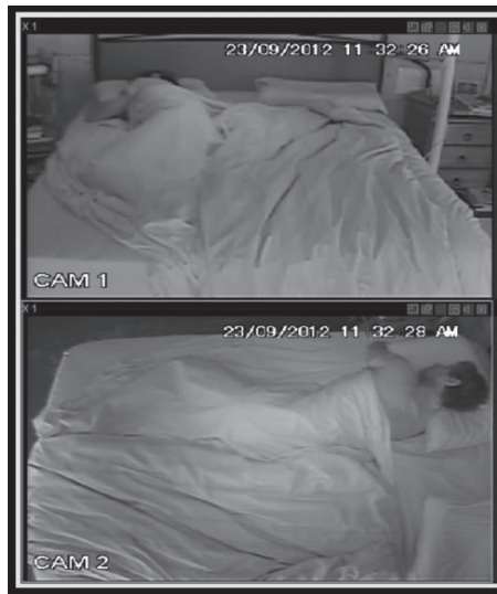
Fig. 3. Visual Quality and Viewing Angles. A criticism of infrared captured images has been picture quality and the subsequent inability to determine sleep posture. For this reason, we selected cameras that provided enough resolution to provide high quality images to discern sleep posture. Furthermore, because pictures have no depth perception, we chose camera alignment that assisted in the determination of relative limb and trunk placement. This picture shows the model in the supported side lying posture, covered by a sheet, from the foot end camera and the overhead camera under infrared light.
