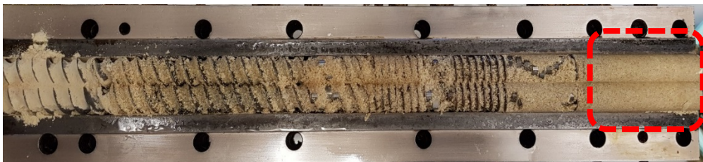
Figure 8.2 The dried seed coat during extrusion cooking blocked die and built-up extremely high die temperature and pressure, resulting in over-torque.
