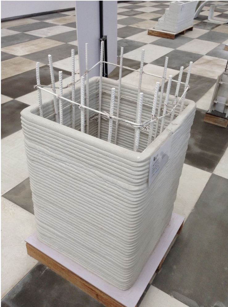
Figure 7. The concrete mould printed by WinSun.
