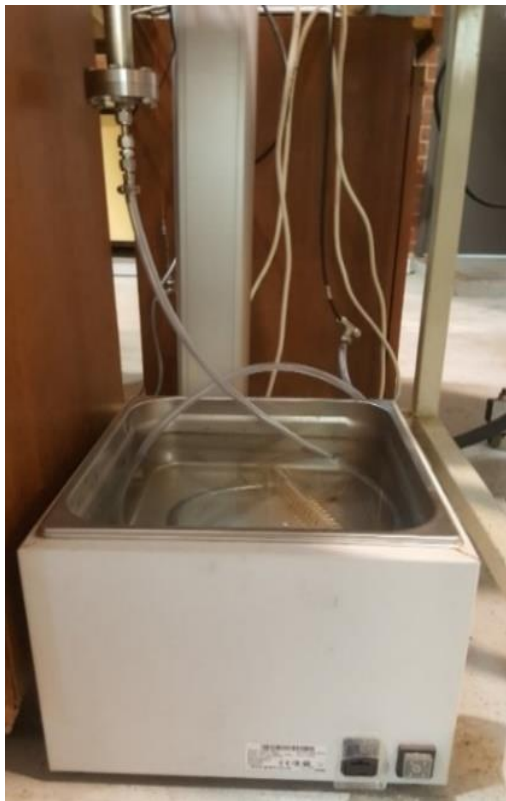
Figure 3. 16 Product gas cooling system
