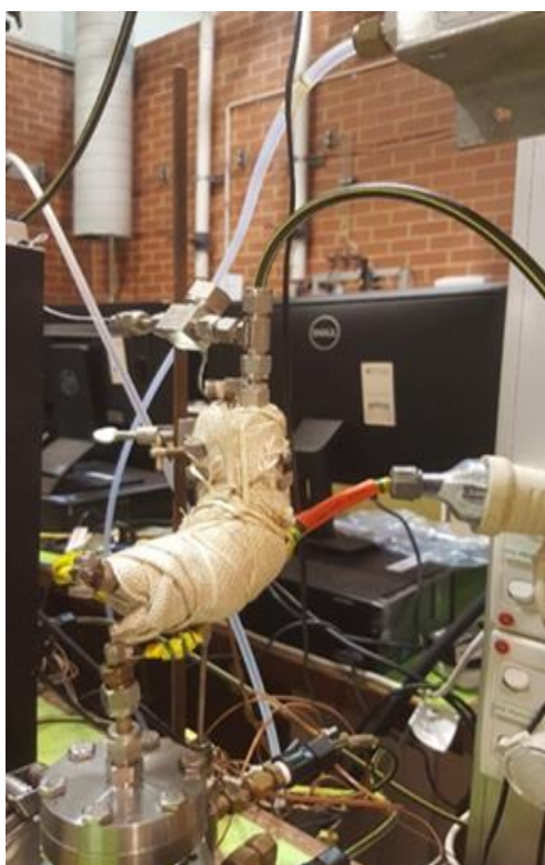
Figure 3. 14 Water addition line (a) LC pump, (b) heated pipeline and (c) heat controller
