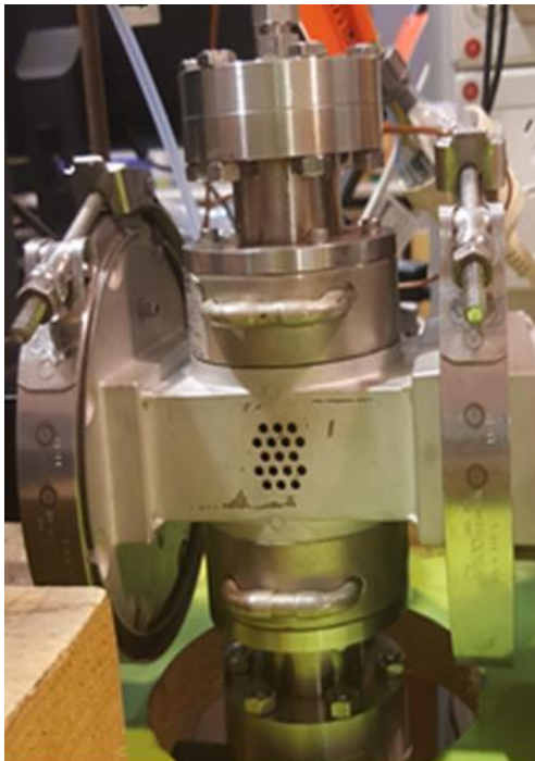
Figure 3. 8 Plasma reactor (a) downstream plasma applicator and (b) water cooling system for plasma reactor
