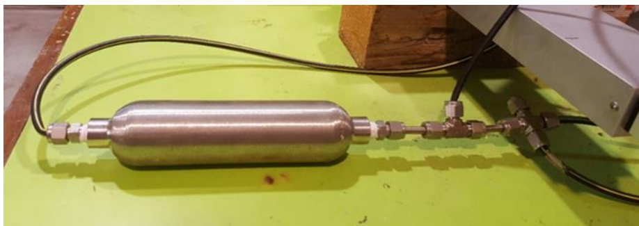
Figure 3. 11 Feeding gas system (a) feeding gases system and (b) gas mixing tank
