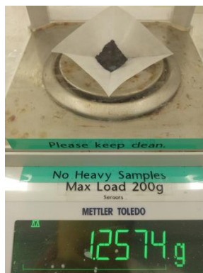
Figure A3-1. Photograph showing a weighing paper containing 1.26 g of single-layer MoS 2 nanosheets.
