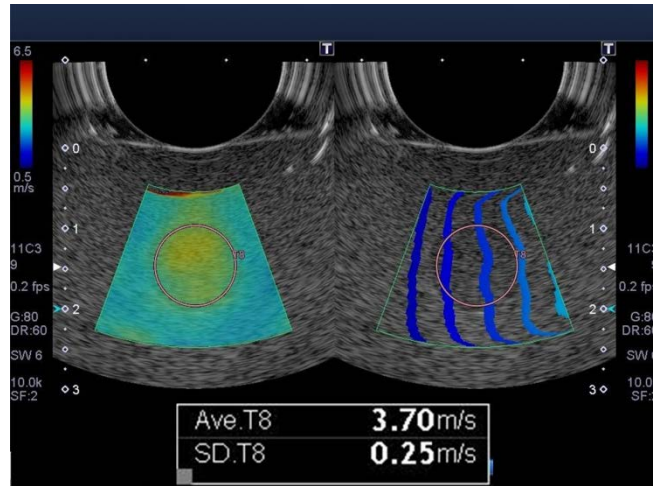
Figure 5.4: Shear wave speed obtained in QA phantom using 11C3 PVT-781VTE endocavity transducer, mean speed of 3.70m/s (SD 0.25m/s)
