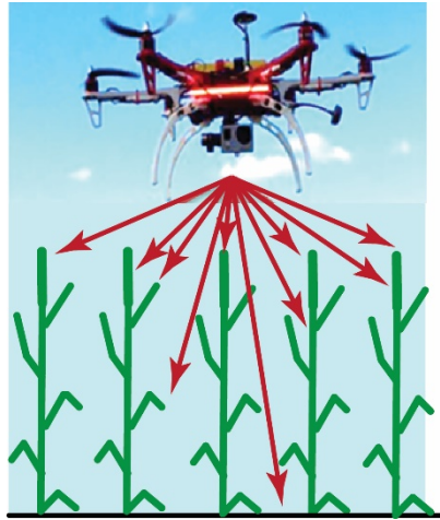
Figure 5: Illustration of potential source of CSM inaccuracy based on image matching.
