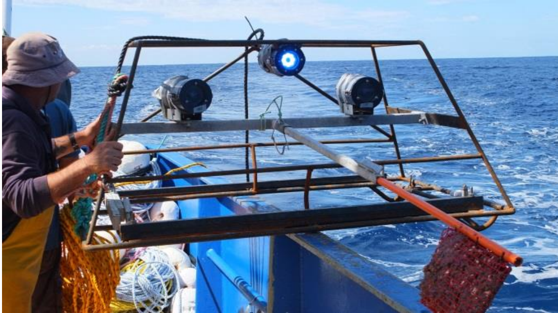
Figure 1.1 Photograph illustrating the basic design of the stereo baited remote underwater video system (stereo-BRUVs) adapted for deepwater deployments.
