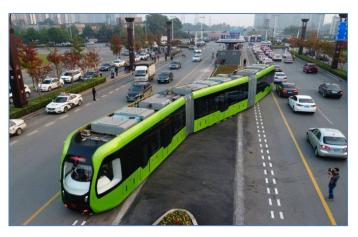
**Figure 1.** The Trackless Tram System developed by CRRC and demonstrated in Zhuzhou, China. Source: Compliments of CRRC Corporation.
