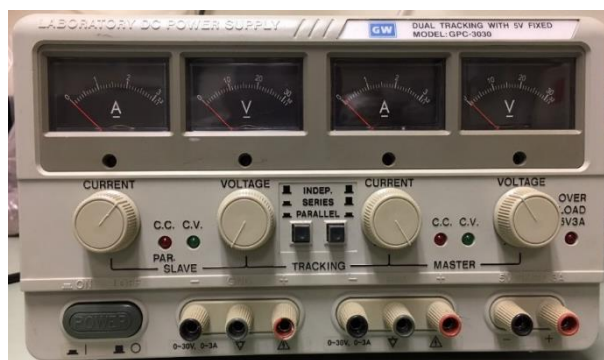
Figure 3. 11 The Power Supply for The Electrical Control Circuits
