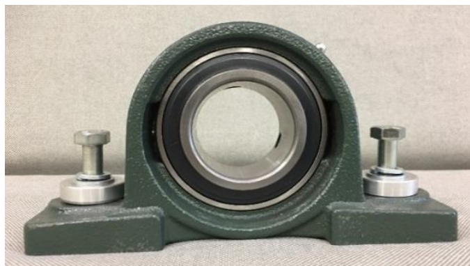
Figure 3. 4 Pillow Blocks with Concentric Locking and Cast-Iron Housing Bearing
