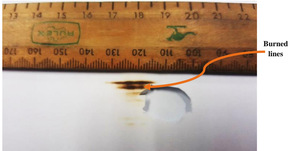
Figure 3. 27 Laser Reflection Sign
