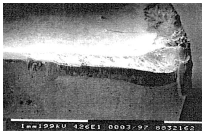
Figure 2. 2 Damaged cutting tool edge in machining Ti-6Al-4V alloy at speed and feed of 100 m/min and 0.25 mm/rev respectively (56)
