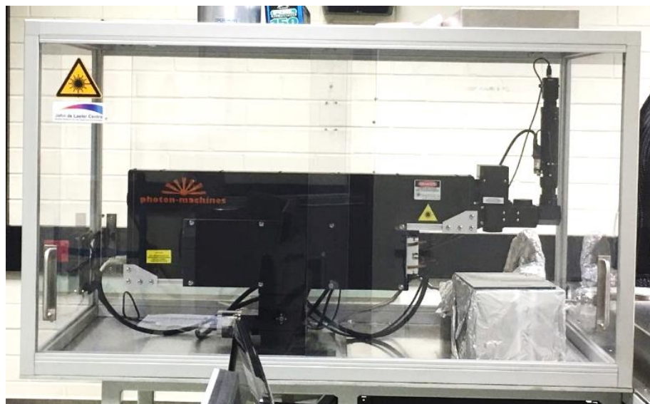
Figure 3. 17 Fusions 10.6 Series installed inside glass container
