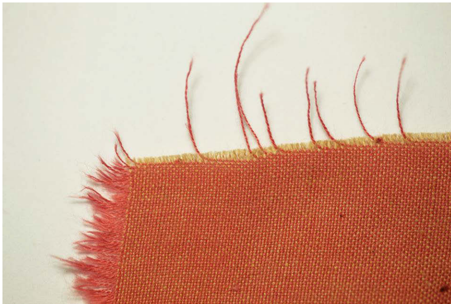
Figure 5. Visual texture: contrasting warp and weft colours in hand woven cotton cloth produced for Bhalo by TSDS (reproduced with permission, Yarwood 2019).
