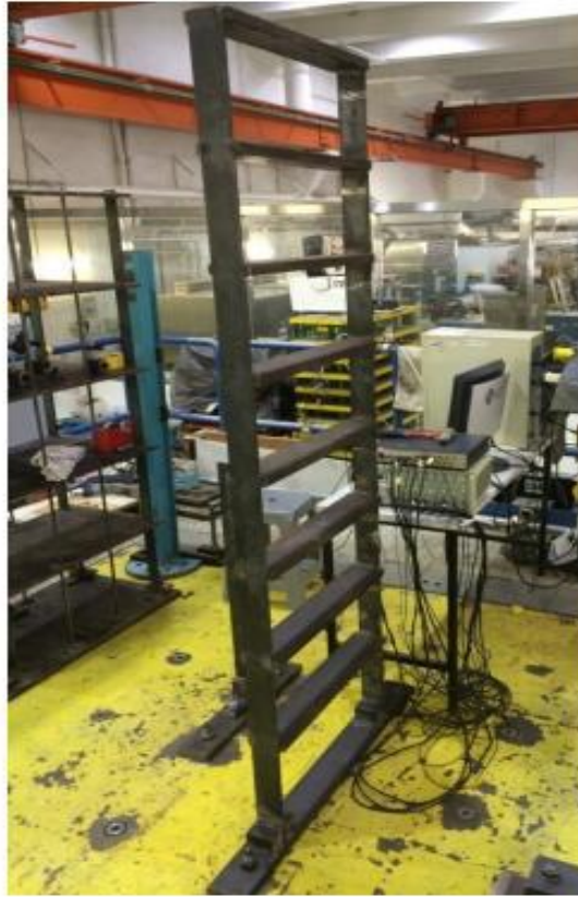
Figure 5-10 A eight-storey steel frame model.
