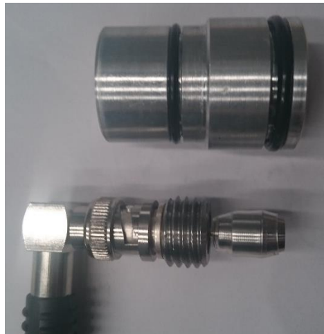
Figure 3-23: Picture of the transducer casing and the steel part that transmits electrical current from a pulser to the piezoelectric crystal (10mm in diameter).
