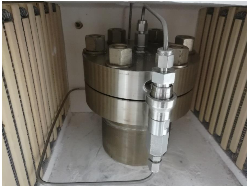
Figure 3-10: Picture of the hydrous pyrolysis cell positioned in the oven.
