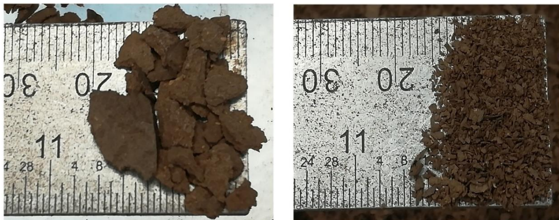
Figure 3-3: Flake particles produced with fresh land OM. The bigger particles (left) were sieved out. The final flake particles (right) range in size between 200 \mu m and 2.3mm, with a low aspect ratio ( <0.25 ).
