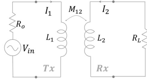
Fig. 2. Traditional transformer model.
