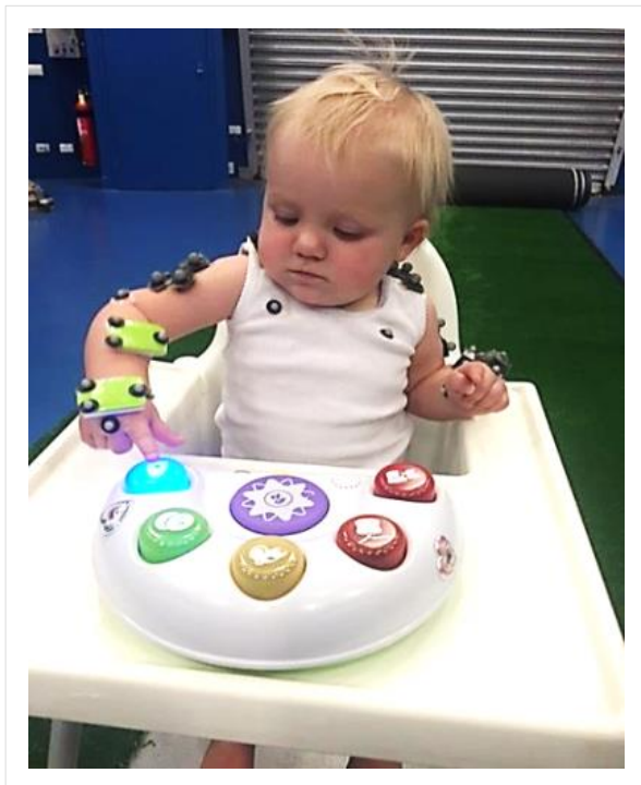
Figure 4.1 The size of Noraxon commercial wearable sensors on the arm of a small child.
