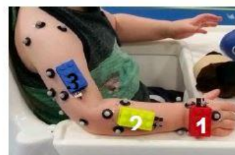
Figure 2: Placement of sensors and 3DMA markers
