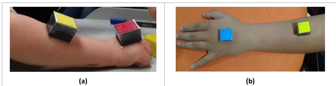
Figure 6.2 Example of the placement of the wearable sensors on the hand and forearm of (a) a young child and (b) an older child.
