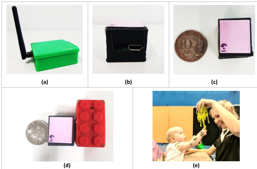
Figure 4.5 V3 wearable sensors; a) receiver dongle the wearable sensors transmit data to; b) external switch and charging usb port; c) size of the wearable sensor compared to a 10c coin; d) size of V3 compared to V1 and 10c coin, and e) V3 wearable sensor on the hand and forearm of a young child.
