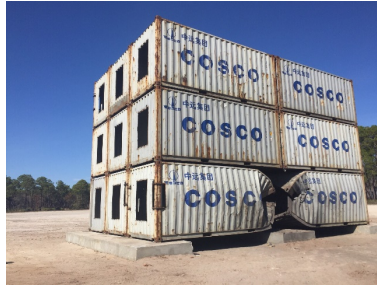
Figure 2.8. Expeditionary CONEX testing for progressive collapse [109]
