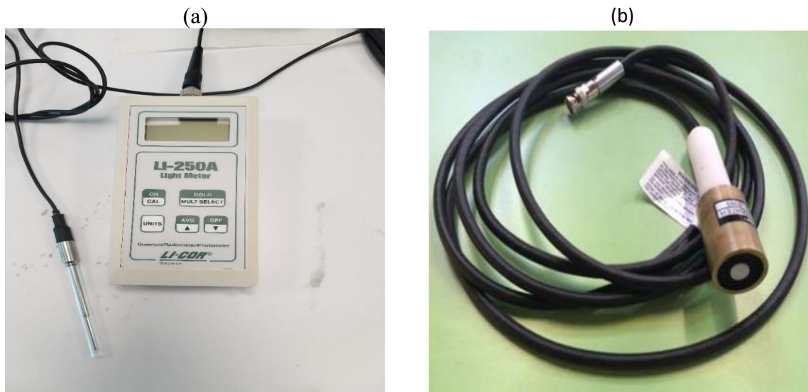
Figure 3. 7 (a) Light meter connected with spherical sensor, (b) quantum sensor
