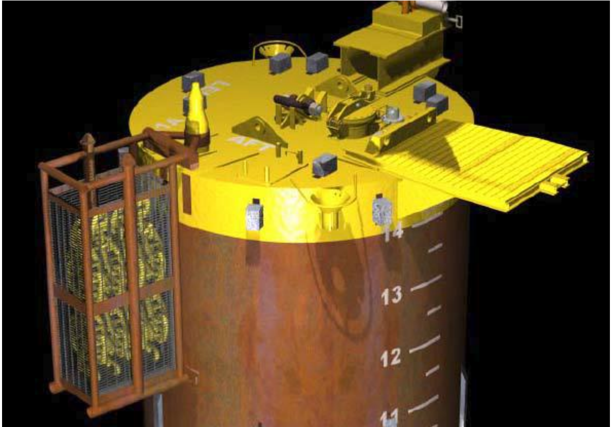
Figure 7-24: Suction pile (Colliard et al., 2006).
