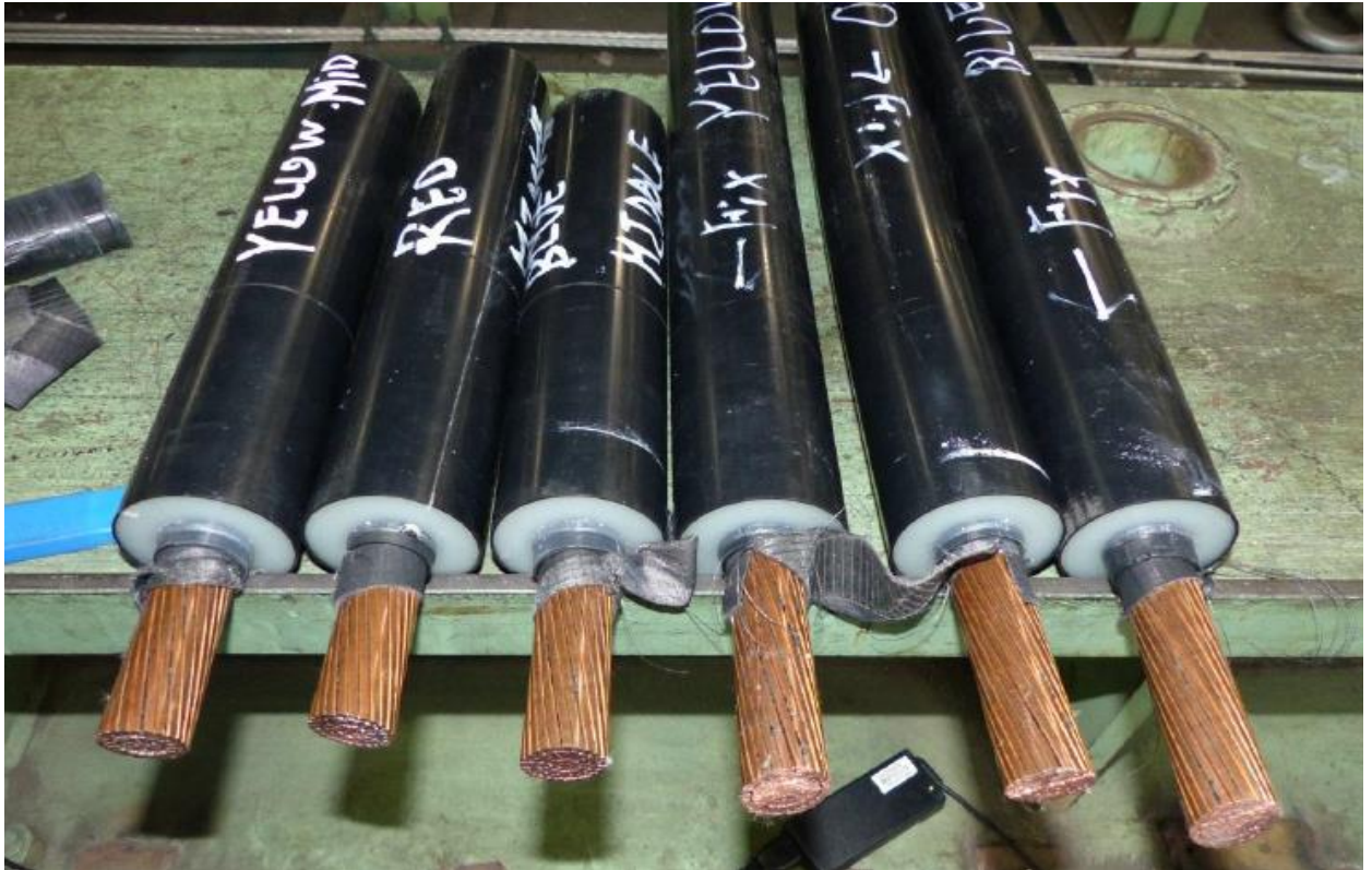
Figure 3-79: Cable conductors after removal of insulation and semi conducting screens.
