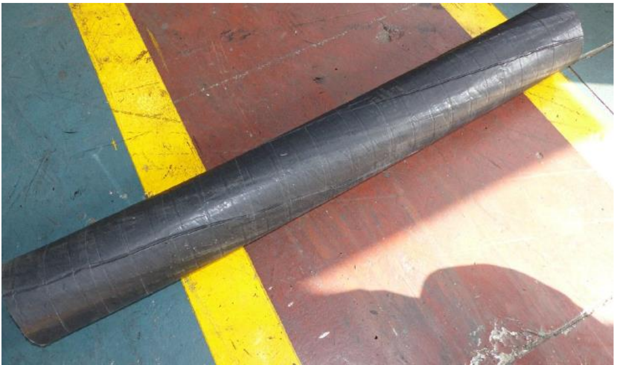
Figure 3-74: Binder tape after removal of the anti-teredo layer.
