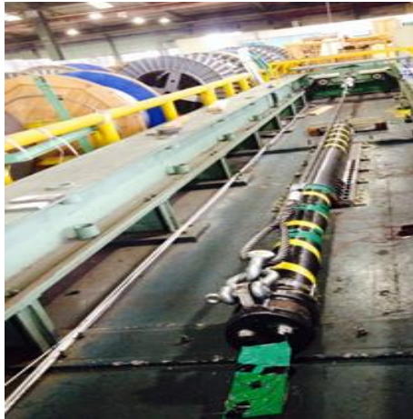
Figure 3-35: Tensile test machine (100 metric tonne capacity).
