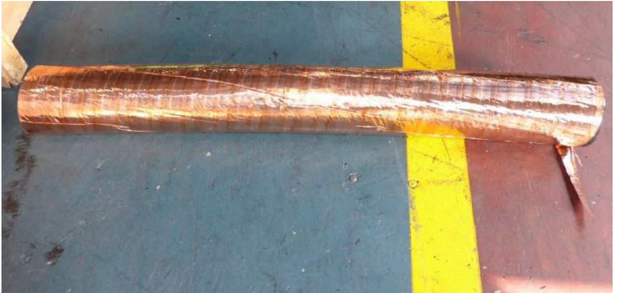
Figure 3-73: Anti-teredo layer after removal of armour bedding layer.
