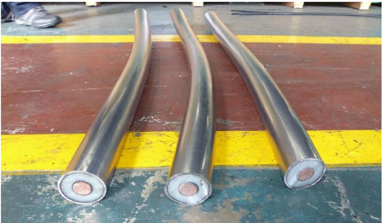
Figure 3-76: Lead sheaths of cable cores after removal of core outer sheaths.
