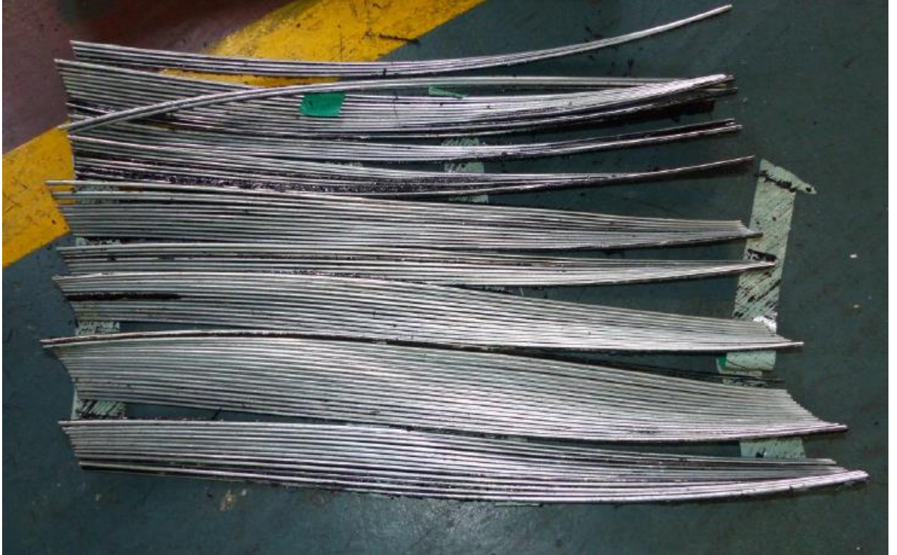
Figure 3-71: Steel armour wires after removal.
