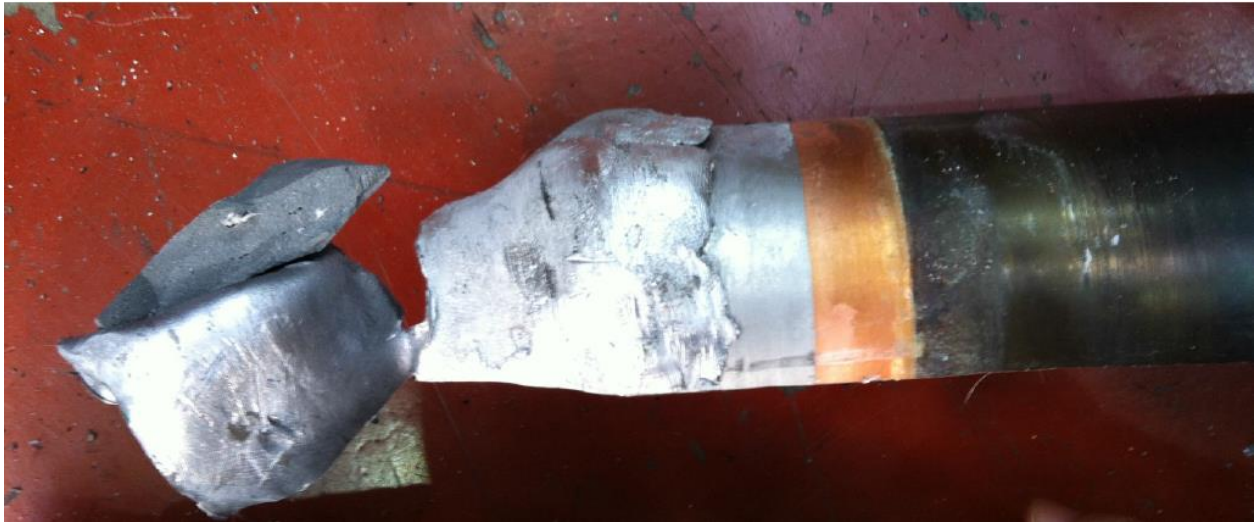
Figure 5-2: Soldering between copper sheath and lead sheath
