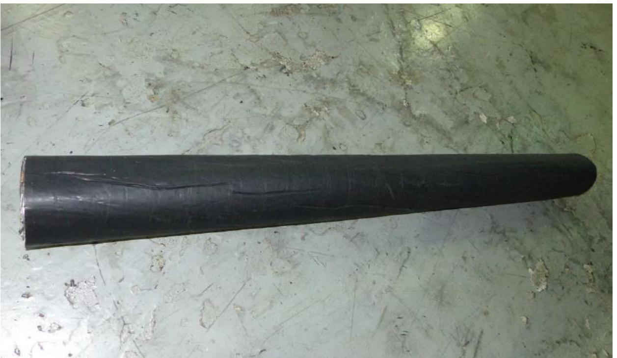
Figure 3-65: Binder tape after removal of anti-teredo layer.
