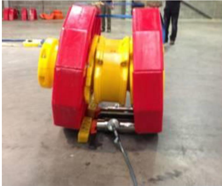
Figure 6-20: Axial load testing of articulated padding assembly.
