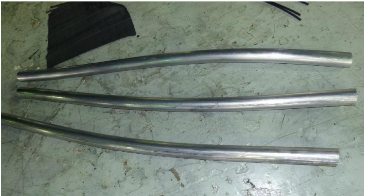
Figure 3-67: Lead sheaths of cable cores after removal of core outer sheaths.
