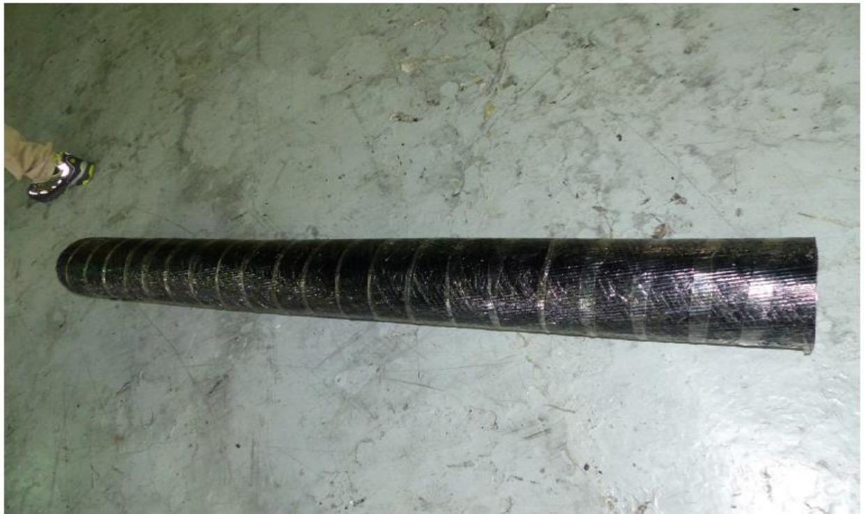
Figure 3-63: Armour bedding after removal of steel armour wires. No deformation or damage was observed.
