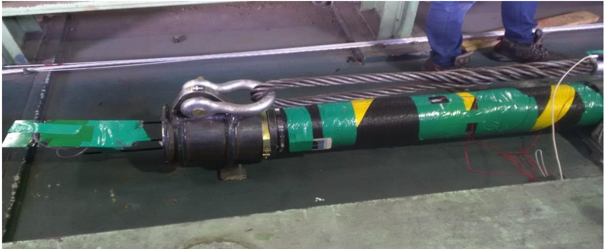
Figure 3-28: Photo of the grip attached to the cable.
