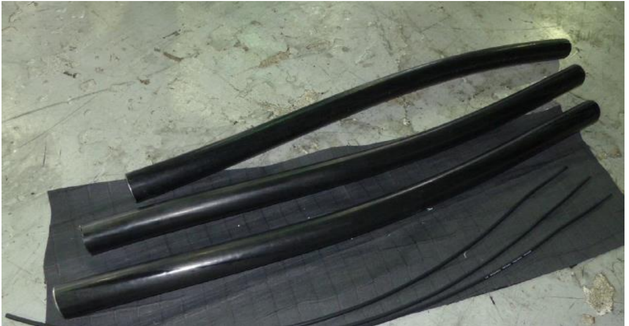
Figure 3-66: Three cable cores and optical fibres.
