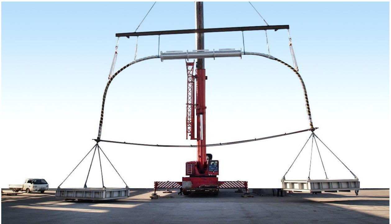
Figure 5-20: Final hanging position for mechanical stress tests (free hanging with additional load).
