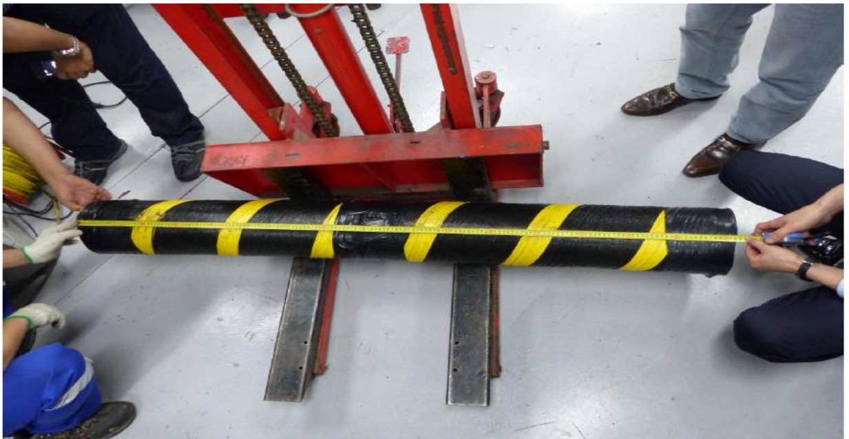
Figure 3-61: Length measurement of cable sample upon completion of pure axial compression test. No deformation or damage was observed.
