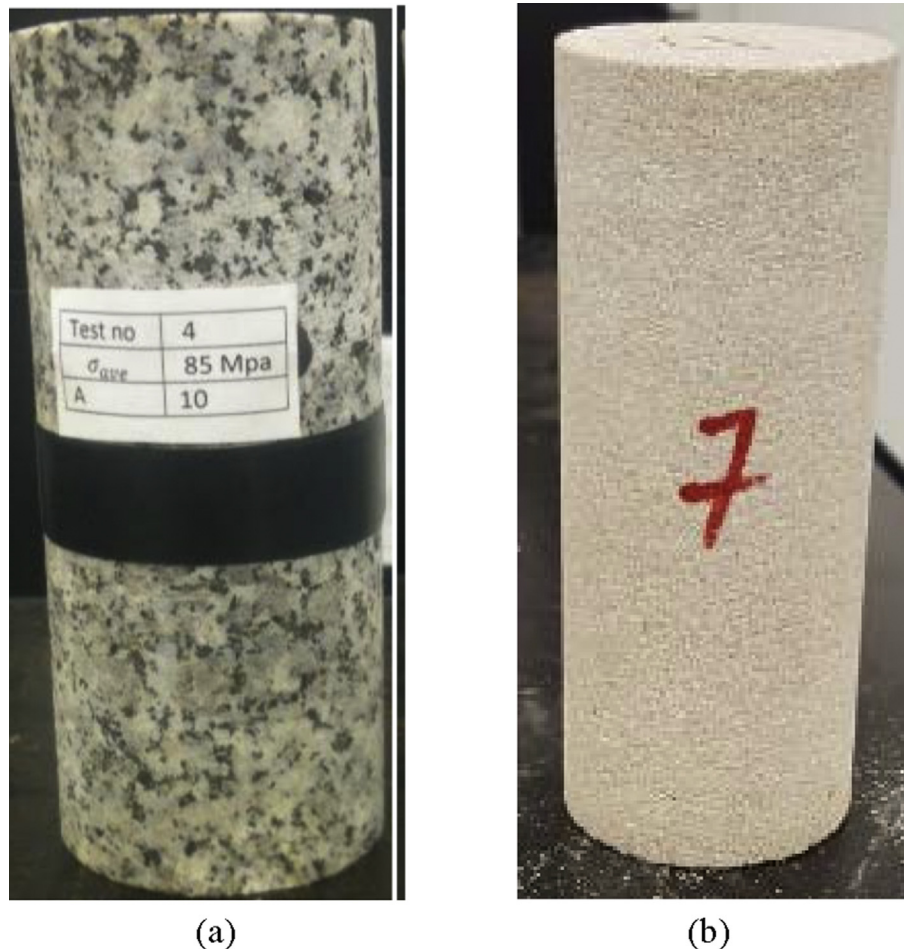
Fig. 3. Typical specimens of (a) granodiorite and (b) sandstone before testing.
