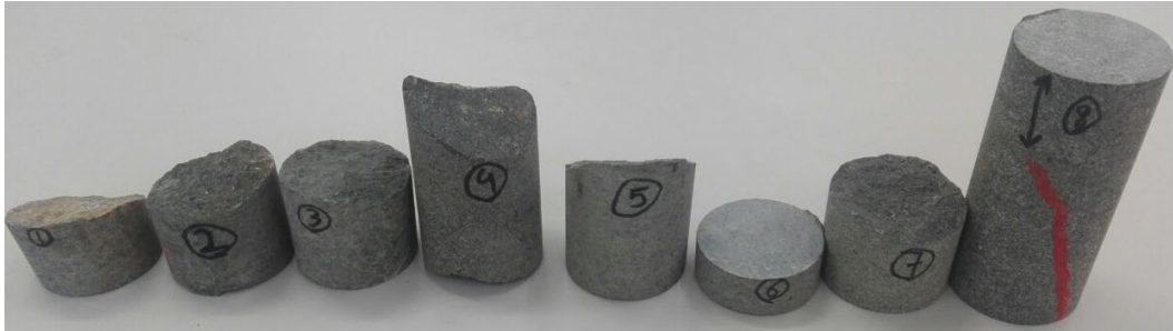
Figure 2.5. Eight rock samples selected for the thin section analysis.
