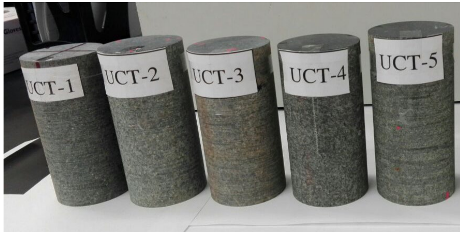
Figure 2.2. Dolerite samples prepared for the UCS testing.
