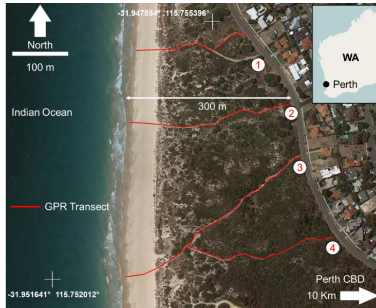
Figure 5.3: Location and orientation of the ground penetrating radar (GPR) transects featured in this paper. Shallow geology is described predominantly Tamala Limestone and Safety Bay sands. Total perpendicular length from the coastline is approximately 300 m.
