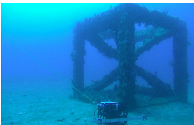
Figure 1. Artificial reef with BlueROV2 and scale bar mounted on a separate ROV
