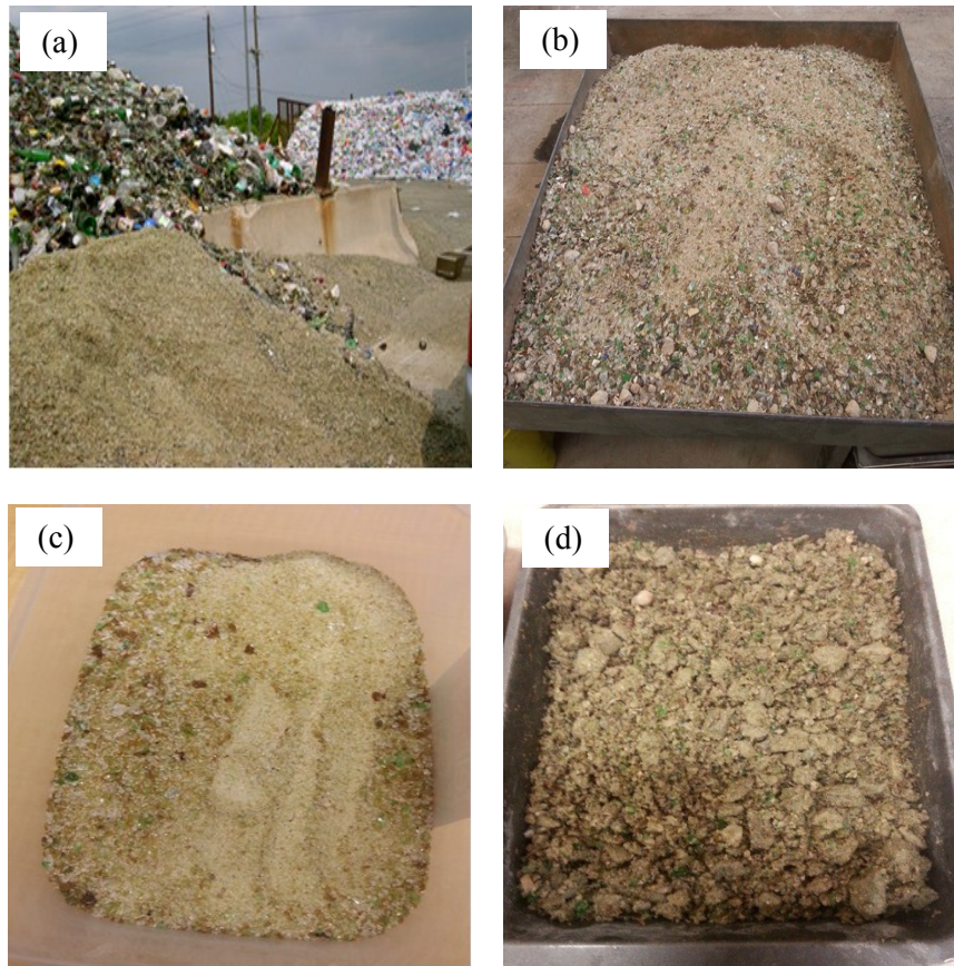
Figure 3.3 a) stockpiles of crushed glass, b) large tray used to mix the materials, c) dry sample of crushed glass, and d) wet glass-rock mixture
