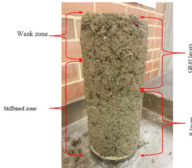
Figure 6.20 Failure patterns observed after RLTT of a 4R+4GR45 sample
