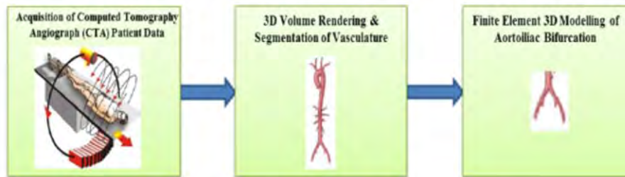
Fig.3 Creation of 3D Solid Model from Patient Specific CTA Data
