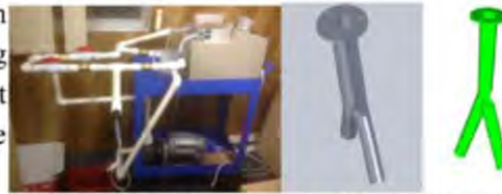
Fig. 7 Benchtop model using 3D printed aorta and pulsatile flow system under development
