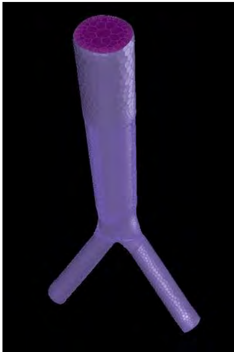
Figure 2-1 Polyhedral Volume Mesh
