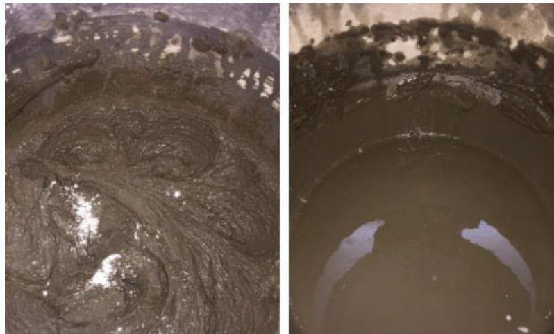
Figure 5-1: Contrasting Mortar Consistencies. (Left– PG2, Right PG4)
