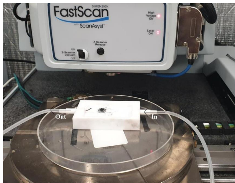
Figure 11. In situ AFM set up, with the liquid pumping in on the right and out on the left
