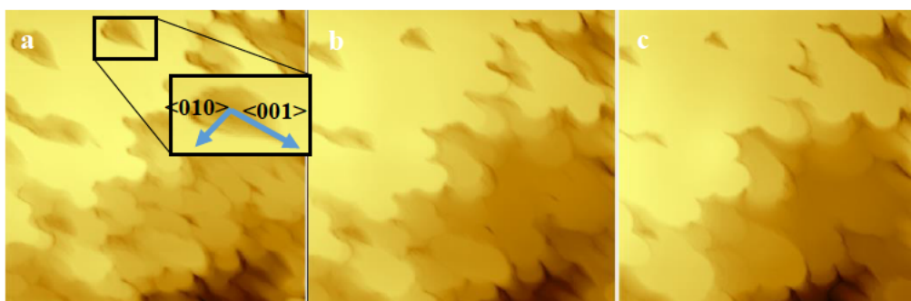
Figure 54. AFM images at different times ((a) followed by (b), followed by (c)) displaying the closing of etch pits and the assignment of growth directions. All images are 5 \mu\text{m} \times 5 \mu\text{m}
