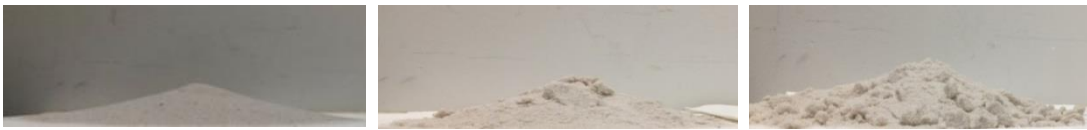
Figure 3.14: (a) Shape of the accumulated grains loose sand (a) Shape of the accumulated grains of the 4 days treated experimental sample (c) Shape of the accumulated grains of the eight days treated experimental sample
