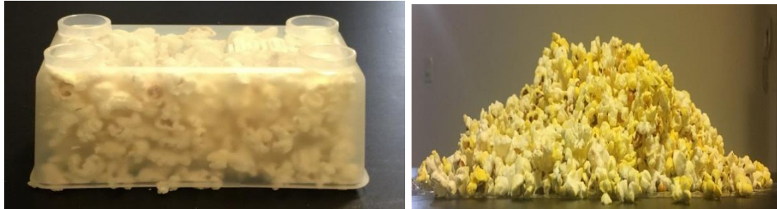
Figure 8.5. The angle of repose study with popcorn (a) pop-cons in the box (b) accumulated shape of popcorns after removing the container
