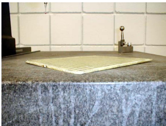
Figure 20: Warpage of a [0/90/0/90/±45/±45/0/90/0/90] E-glass/epoxy panel
