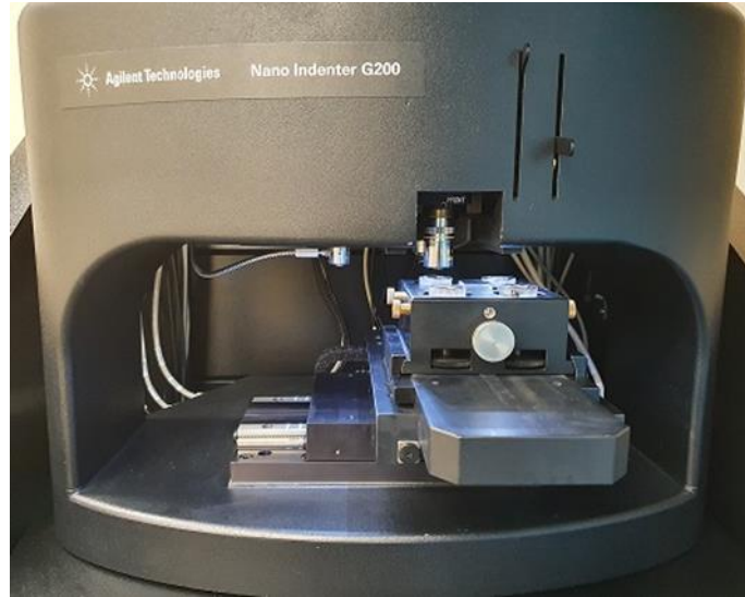
Fig. 5.1 Nanoindentation test setup in Agilent Nano Indenter G200
