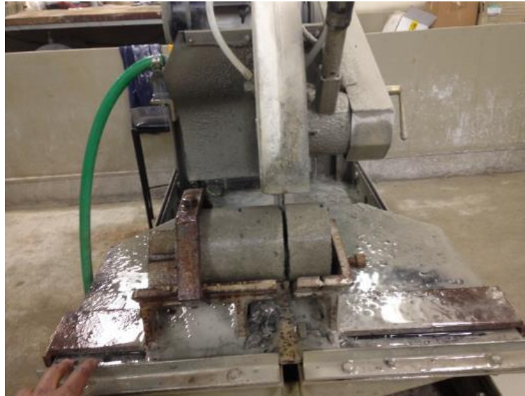
Fig. A.3 Cutting concrete cylinders in 50 mm discs
