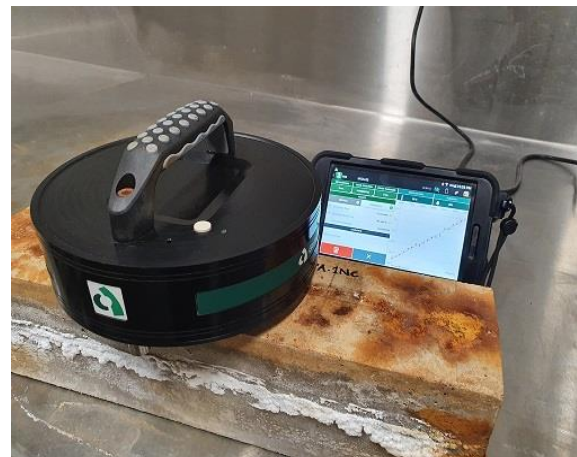
Fig. A.7 (a) Test setup (b) Data collection of Corrosion test of concrete samples
