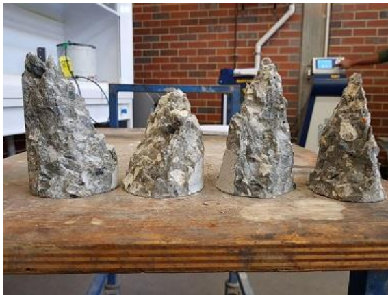
Fig. A.2 Failure pattern of control concretes (left) and concrete with nano materials (right) after compression test
