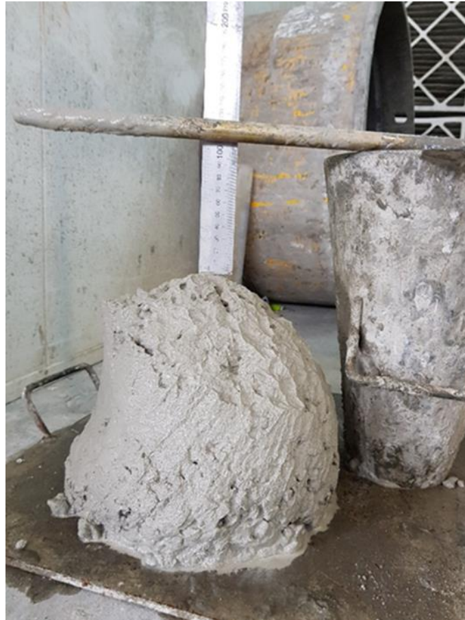
Fig. 8.1 Slump test of a concrete mix
