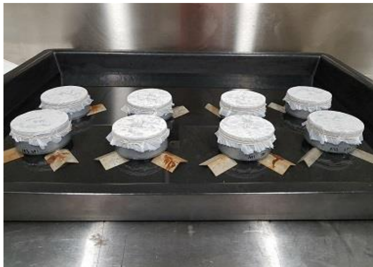
Fig. A.4 Sorptivity test of concrete
