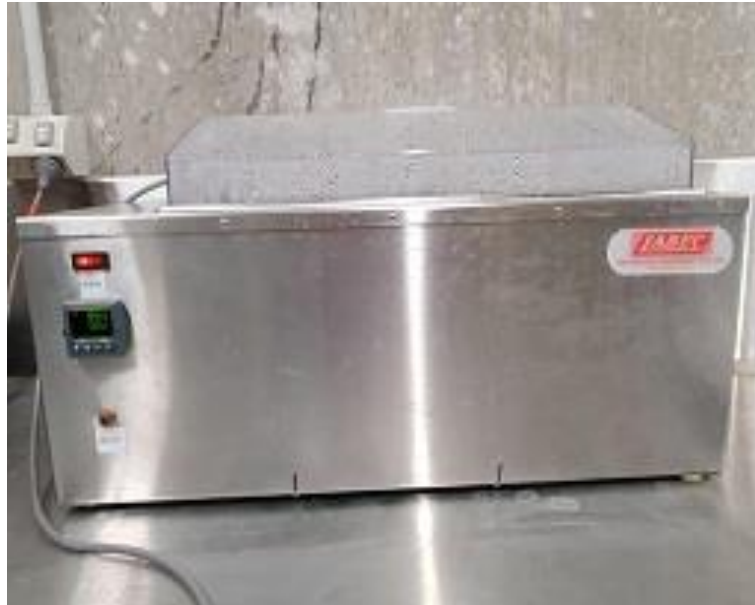
Fig. A.6 Boiling samples in a water bath for VPV test
