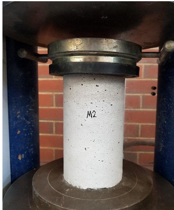
Fig. A.1 Compression test of a typical concrete cylinder
