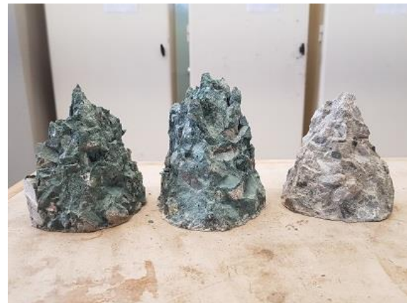
Fig. A.2 Failure pattern of control concretes (left) and concrete with nano materials (right) after compression test
