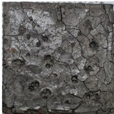
Figure 2. Corrosion cracks on surface of a concrete sample immersed in sodium sulfate solution of 8% concentration for 250 days.
