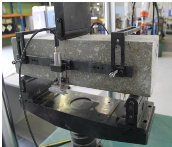
Figure 5-6. Experimental set up for determining load-CMOD relationships
