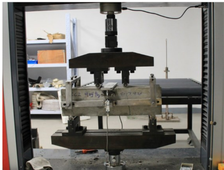
Figure 5-7. Experimental set up for determining load-deflection relationships
