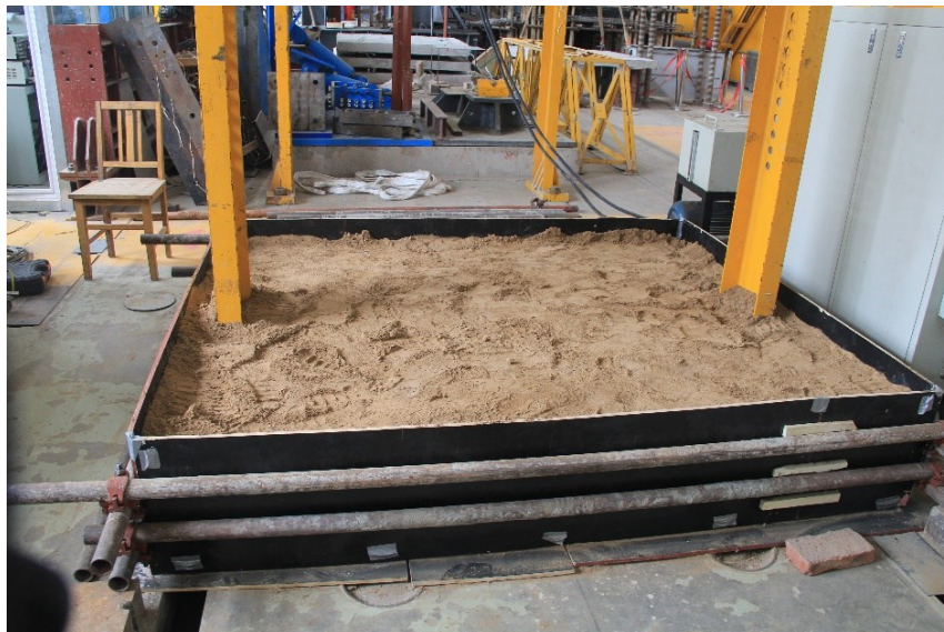
Figure 5-3. The compacted and low-plasticity soil in the soil containment box
