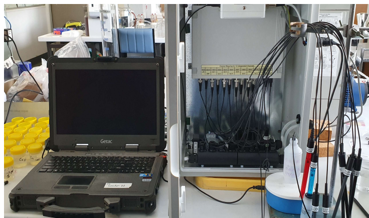
Figure 7-2 Ion-selective electrodes for water chemistry measurements during spontaneous imbibition tests [58].
