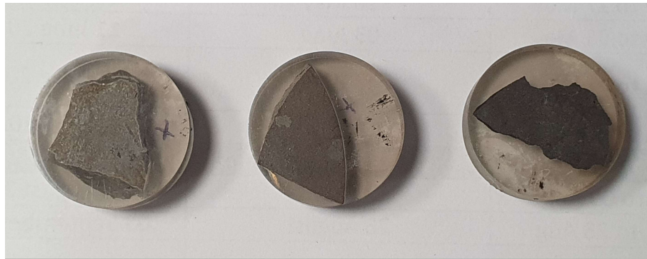
Figure 10-1 Shale rock specimens mounted with resin that rich in (from left to right) calcite (TH-1), clay (mainly illite, TH-5) and quartz (TH-6), respectively.
