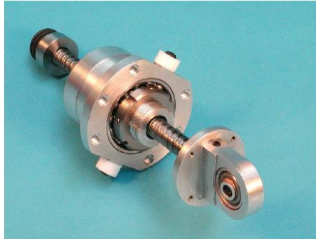
Figure 1-4 Ball-screw inerter developed by Papageorgiou et al. [24]
