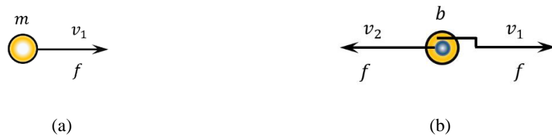
Figure 1-2 One-terminal mass element and two-terminal inerter element
