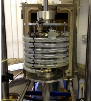
Figure 1-10 Helical fluid inerter developed by Domenico et al. [29]
