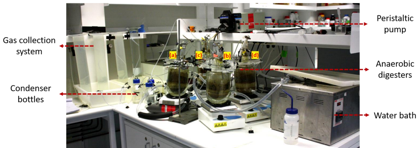
Figure 3.5: Two-stage anaerobic digestion set-up used in the current thesis work. Reactors (a) and (c) are connected semi-continuously in two-stage set-up. Similarly, reactors (b) and (d) are connected to form a control two-stage set-up. Reactors (a) & (b) serve as phase-I and reactors (c) & (d) are operated as phase-II digesters. The reactors are maintained in their respective temperature conditions by water circulation through a jacket heating system.
