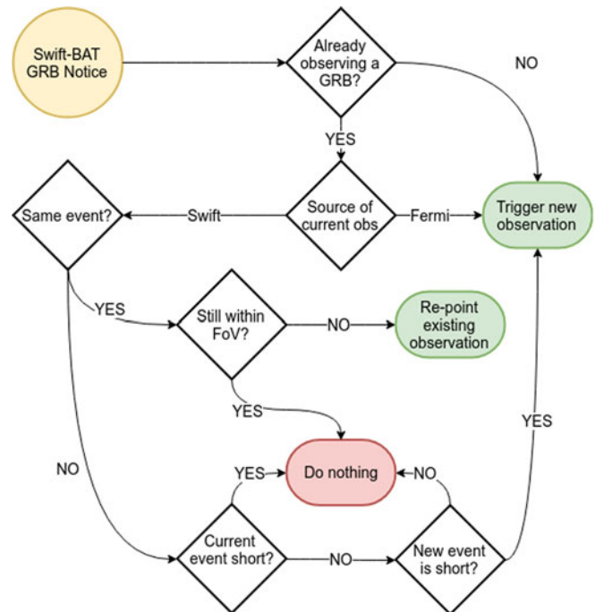
Figure 4. Logical flow for receiving a Swift GRB alert. The outcomes are either to trigger a new observation, update the current observation (green), or to not observe (red).
