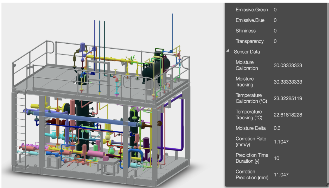
Figure 21. Property Panel of a section of pipeline in web-based BIM model viewer
