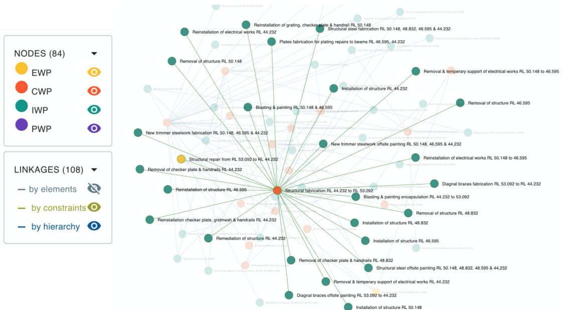
Figure 40. The CWP “Structural fabrication RL 44.232 to RL 53.092” as linked to twenty-six IWPs based on the spatial data and hierarchy of work packages
