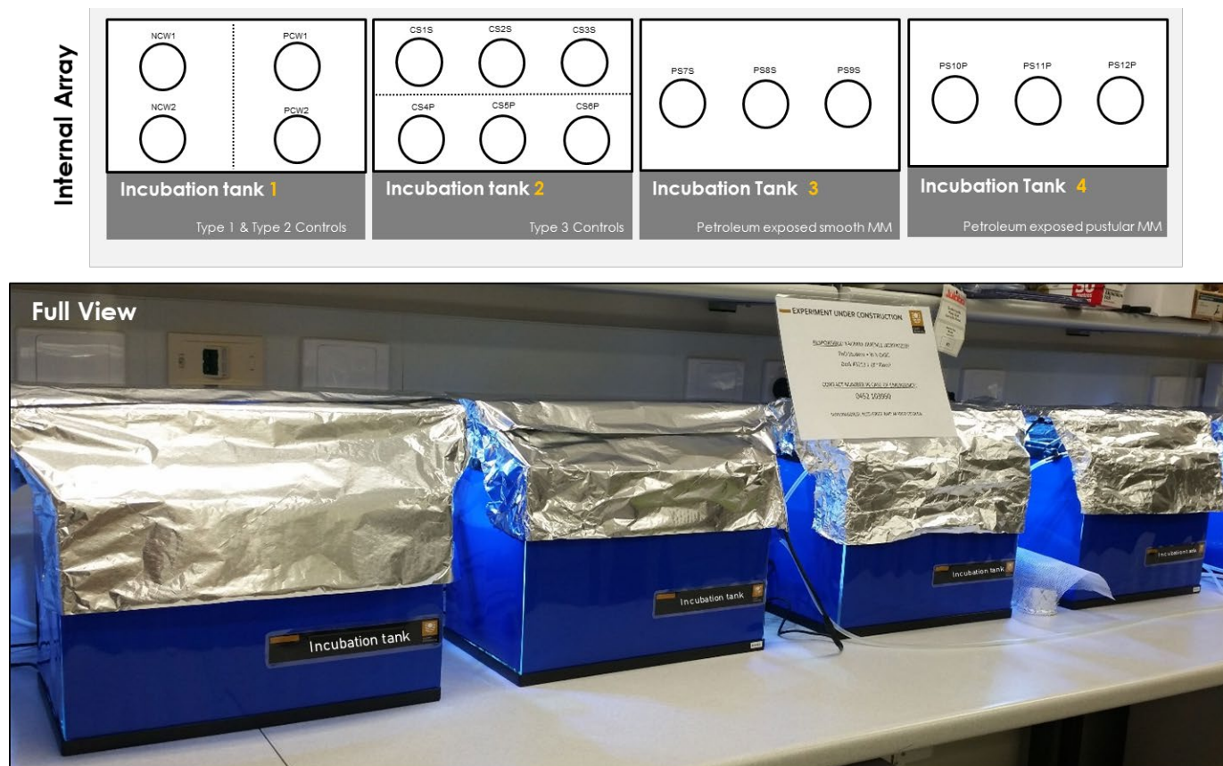
Figure A2.2. Incubation tanks configuration. The top image illustrates the internal array of microcosms in each incubation tank. Photograph on the bottom shows how they were maintained and protected under laboratory conditions. For details of types of microcosms and the nomenclature used see Figure 2.3 and Figure 2.4 .
