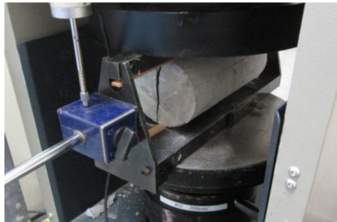
Figure 3.5: Splitting tensile test
