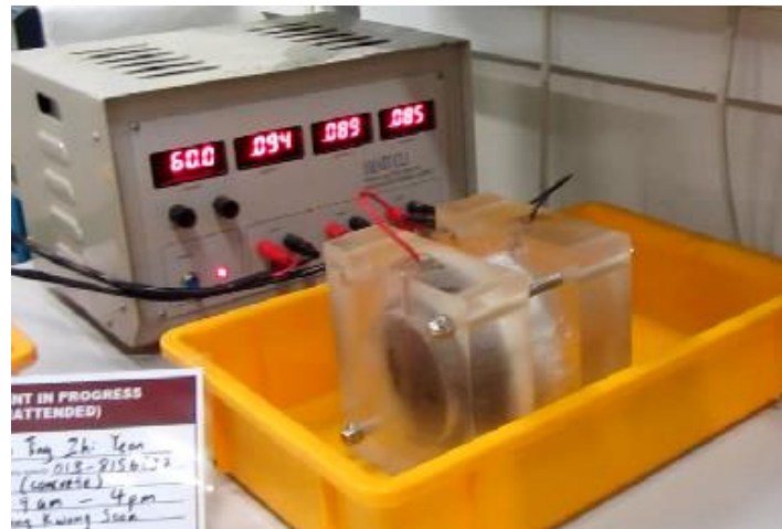
Figure 3.7: Rapid chloride ion penetration test
