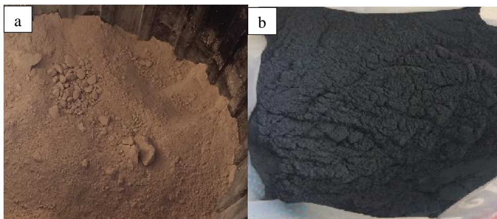
Figure 4.2: (a) FA sample and (b) SF sample
