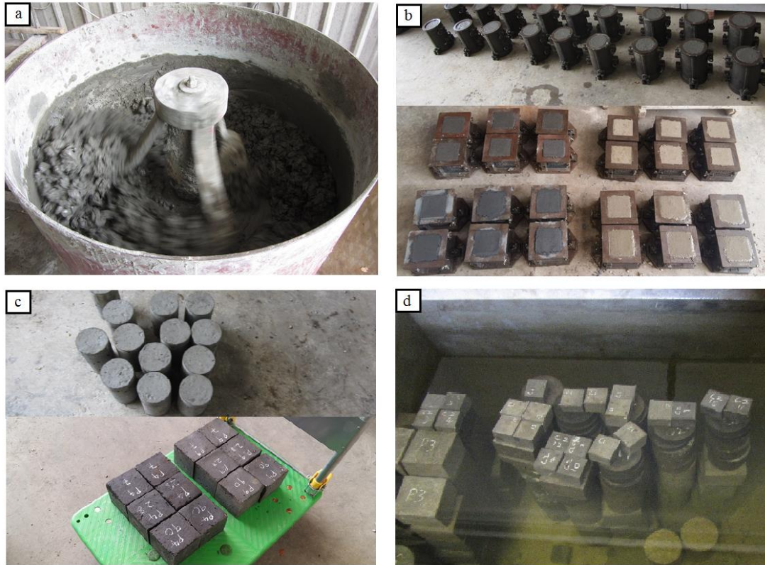
Figure 3.2: Concrete specimens (a) mixing, (b) casting, (c) demoulding and (d) curing
