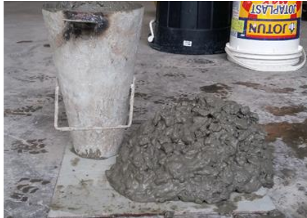
Figure 3.3: Concrete slump test
