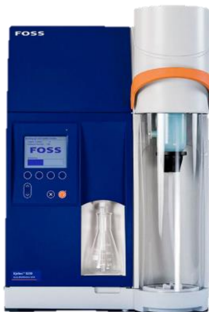
Figure 3.1 – Foss Kjeltac 8200 Distillation Unit, taken from Foss Brochure (2018)
