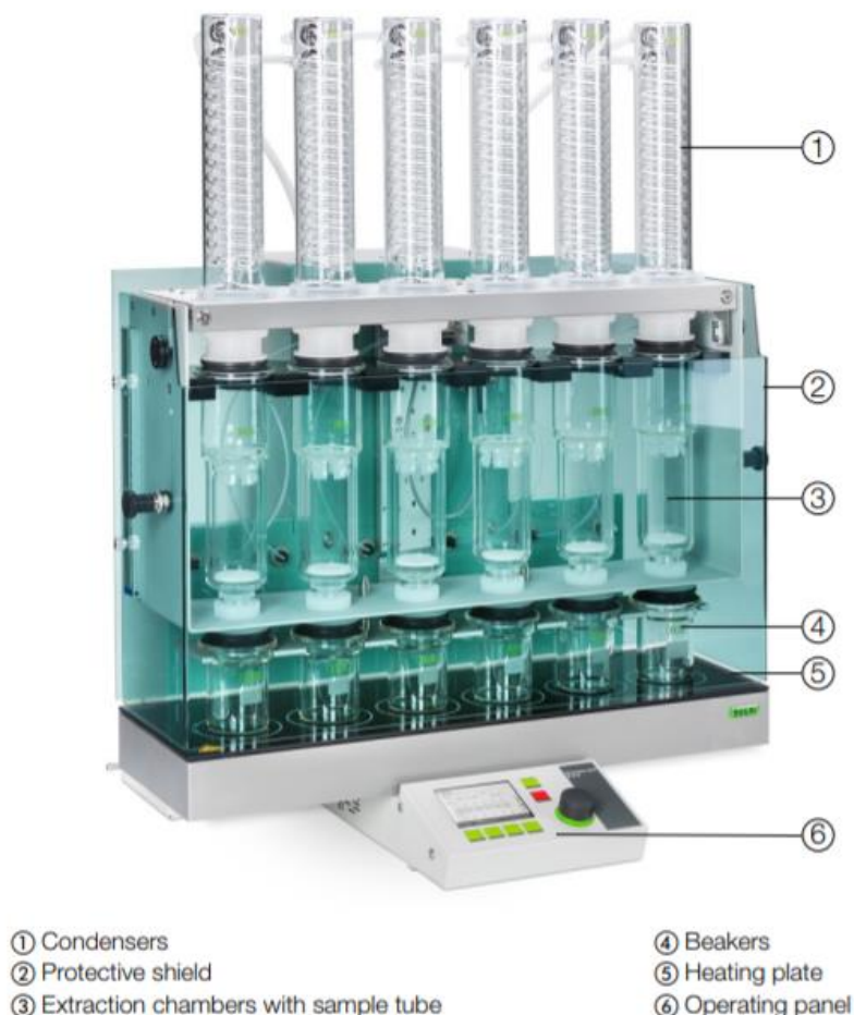
Figure 3.2 - Buchi Extraction Unit E-816 ECE, taken from Operation Manual (Version A, 2015).
