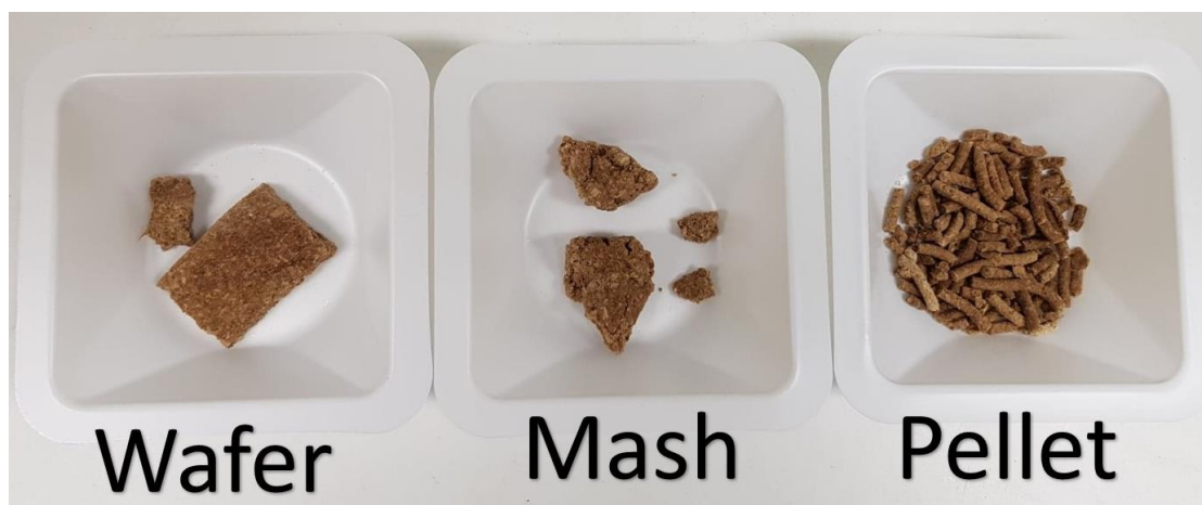
Figure 6.1 – Crustacean feed manufactured into 3 experimental shapes using Poultry by-product meal as a Fish meal replacement.
