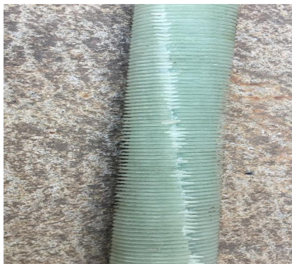
Fig. 2-19. The failure of CFRP bolts when being prestressed with a high level using a torque wrench.
