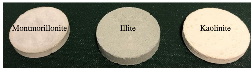
Figure 3. 8 Compacted montmorillonite, illite and kaolinite
