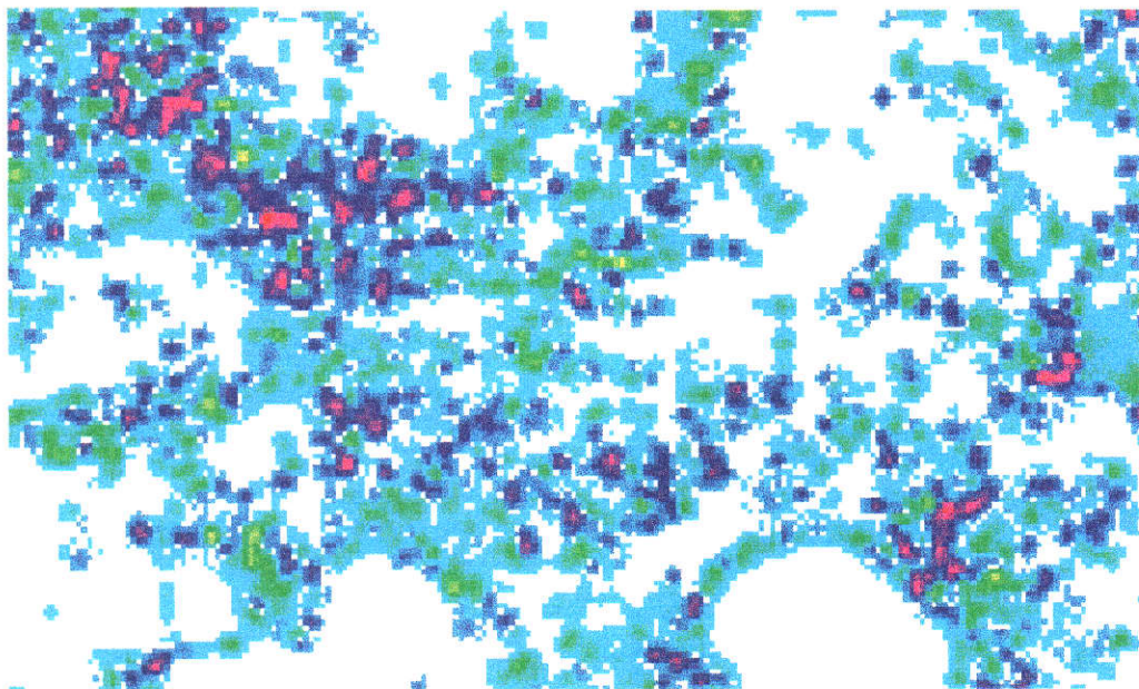
Figure 8.5: Difference of the images shown in figures 8.3 and 8.4. The figure is coloured red, representing a relatively large positive difference of approximately 0.25, through pink, blue, cyan, and green, which represents a relatively large negative difference of approximately 0.15. White represents no differences.
