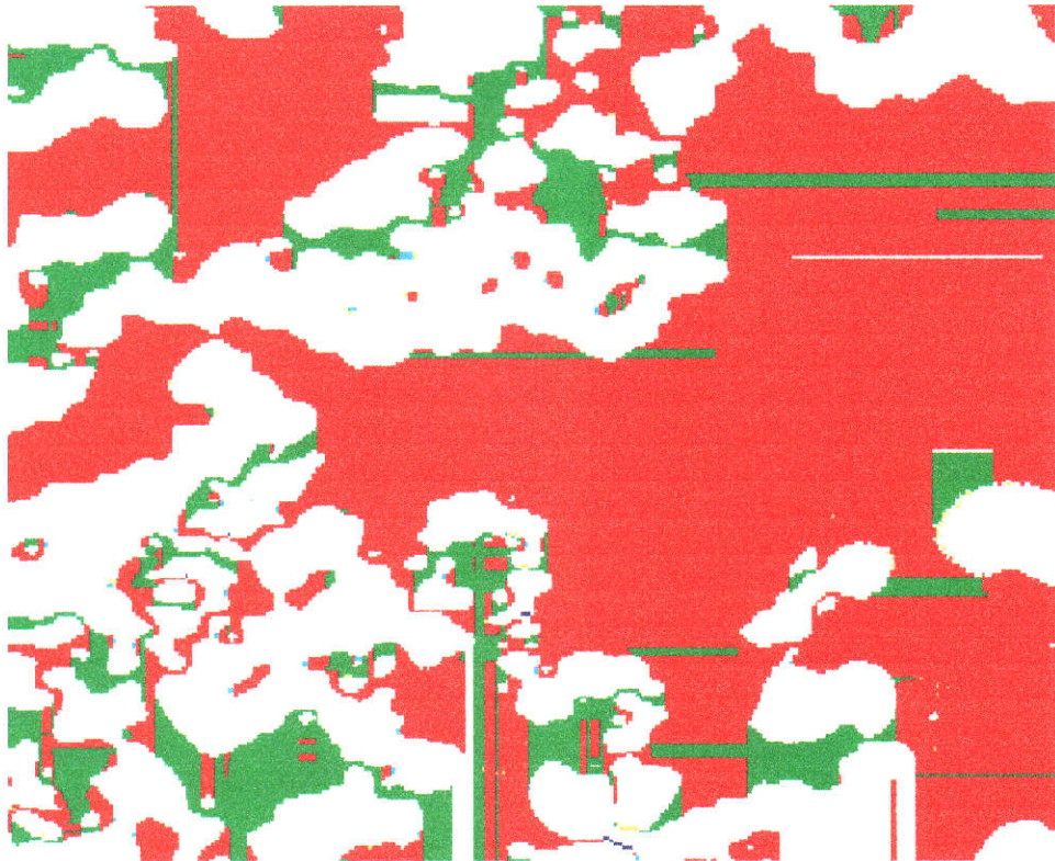
Figure 5.15: Flat area classification of the broad-scale DEM produced using the algorithm described by Chorowicz et al. (1989). Flat hill tops and ridges, flat valleys, flat inflexions and non-flat regions are coloured green, red, blue and white respectively.
