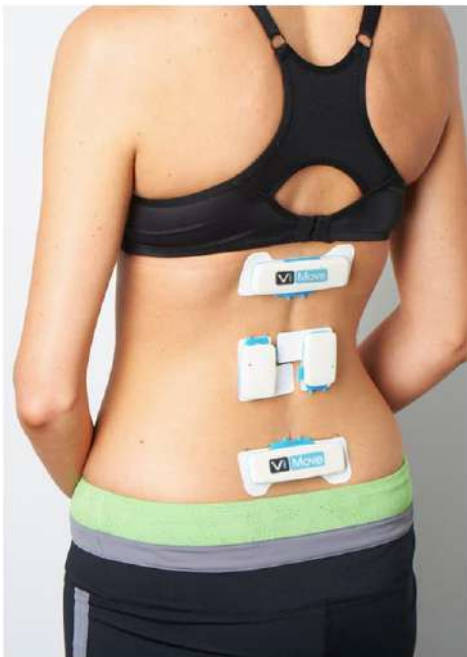
FIGURE 1 The ViMove v5 wireless wearable sensor system to collect kinematics and muscle activity
