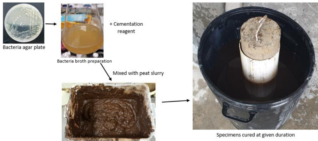
Figure 3.8. Sample preparation flow of peat samples treated with MICP (bacteria and cementation reagent).
