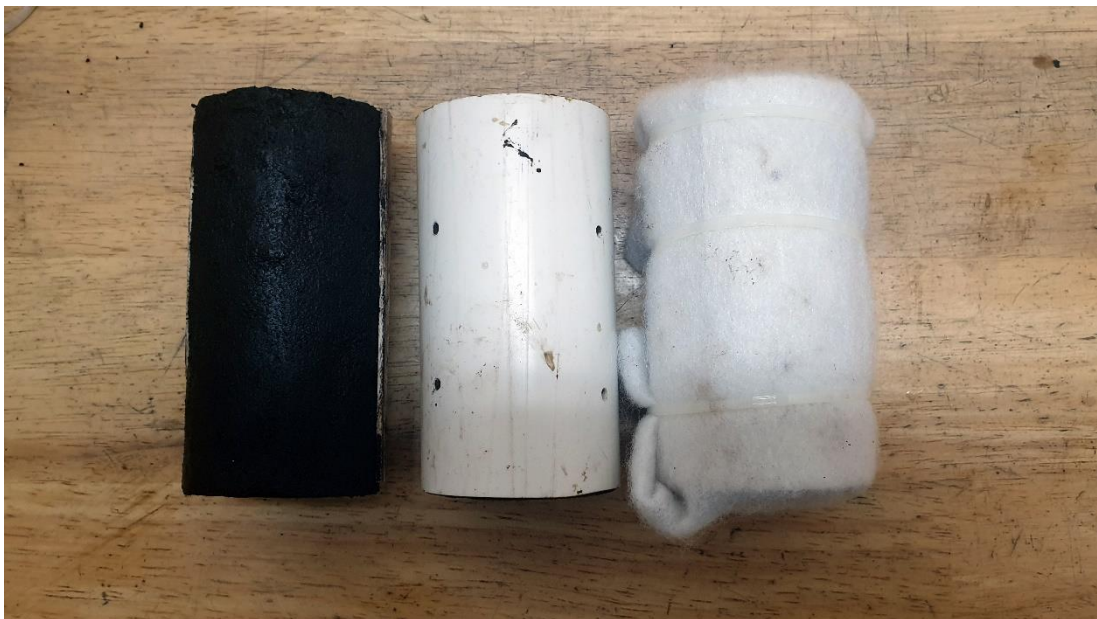
Figure 3.9. Stabilised peat sample trimmed and placed in a PVC tube with holes and wrap with geotextile before submerged to peat slurry and distilled water.
