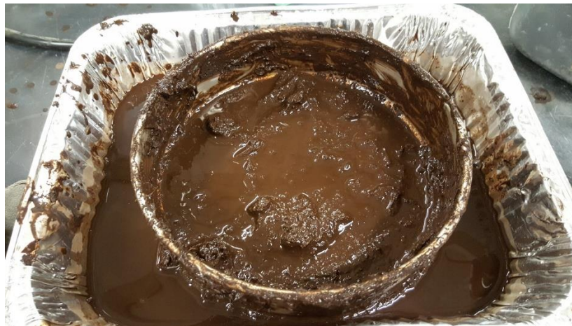
Figure 3.5. Wet sieving of peat. Peat passing 2 mm sieve were used.
