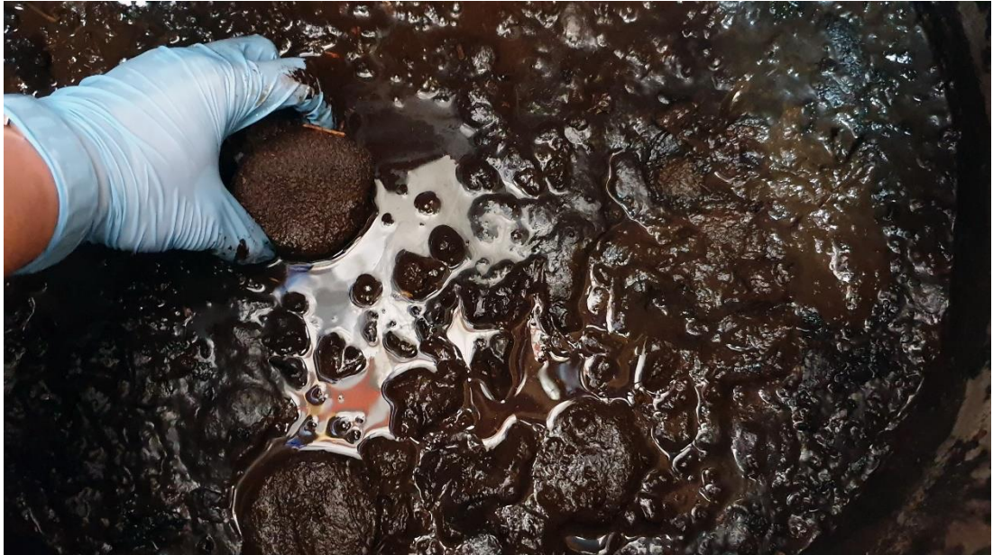
Figure 3.10. Peat samples were placed vertically into a tank containing peat slurry and submerged up to 90 days.
